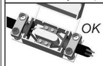
CONNECT CABLES BY INSULATED TERMINAL BOX WITH CABLE CLAMPS ON BOTH SIDES (not included)
